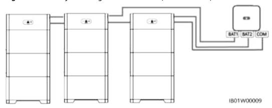
Figure 6-20 Battery cascading cable connection (four batteries)
