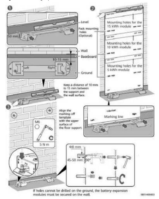
Figure 5-4 Installing expansion bolts
