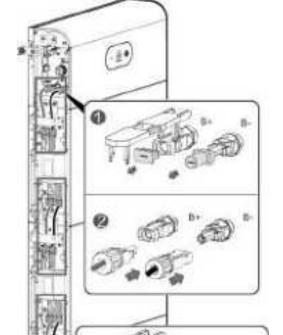
Figure 6-5 DC power cable connection inside the battery
