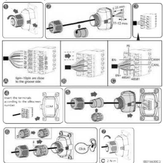
Figure 6-22 Cascading communication terminal
