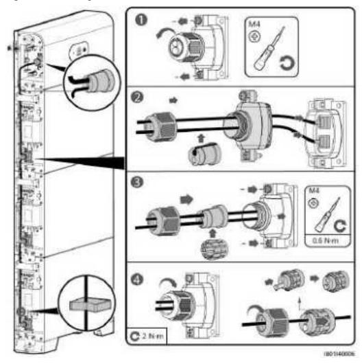
Figure 6-7 Securing With Screws
