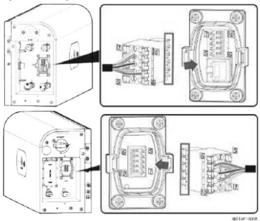
Figure 6-16 Inserting the terminal
