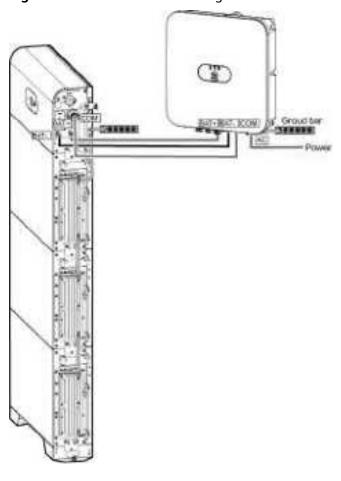
Figure 8-3 Cable connection diagram
