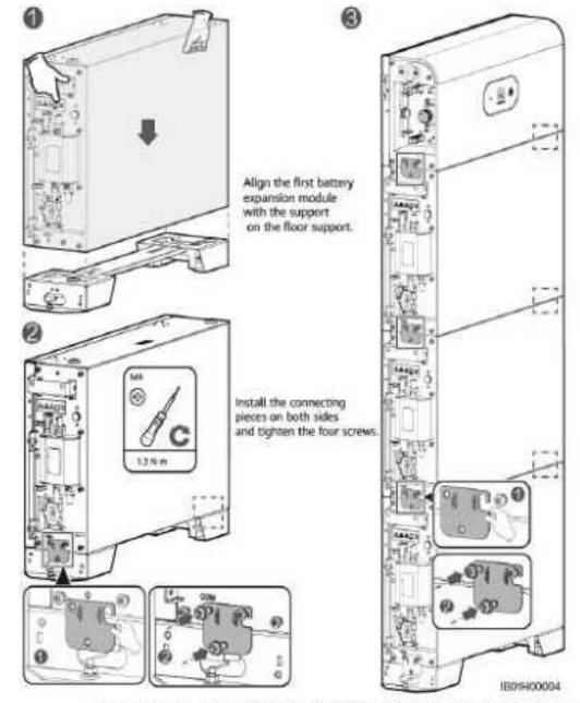
Figure 5-5 Installing the battery expansion modules and power control module
