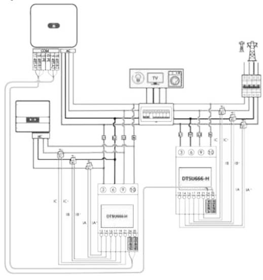
Figure 4-19 Power meter cable connections for SUN2000-(3KTL-10KTL)-M1
