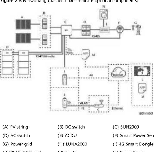
Figure 2-5 Networking (dashed boxes indicate optional components)
