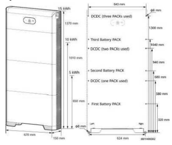
Figure 5-2 Floor-mounted installation dimensions
