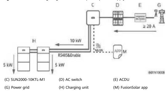
Figure 8-1 Networking diagram for three-phase power supply scenario
