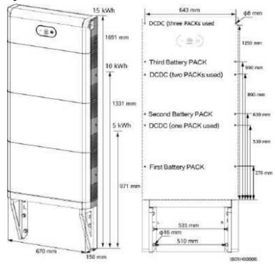
Figure 5-7 Wall-mounted installation dimensions
