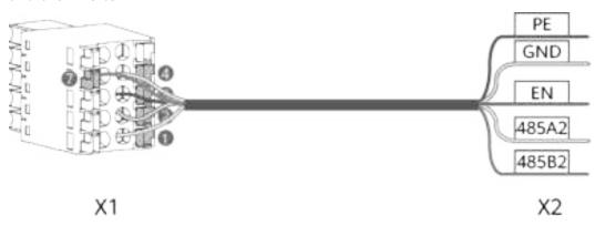
**Table 6-2** Signal cable connection (purchased from the supplier, type 1) between the battery and the inverter
