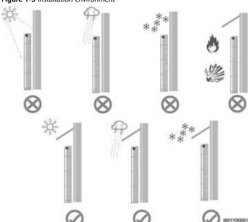
Figure 1-3 Installation environment
