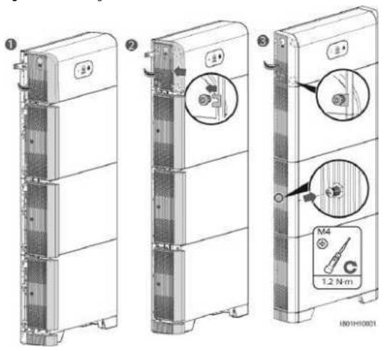
Figure 6-23 Installing the cover
